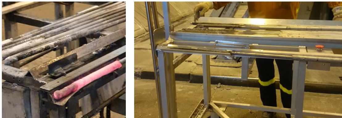
Figure 3. Bath metal dip trolley. Left: interface and slide rule, Right: side view.
