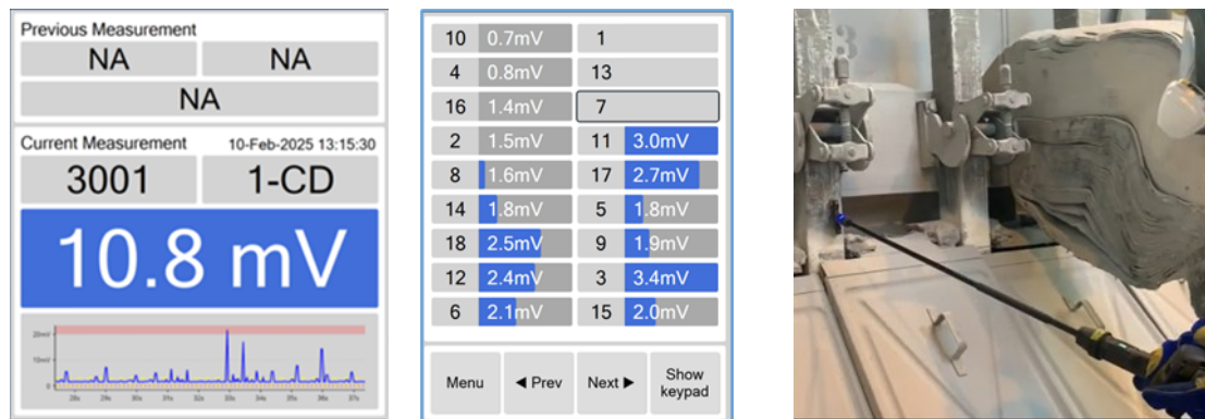
Figure 1. Anode current distribution. Left: User interface, Right: Rio Tinto CAT CD probe.
